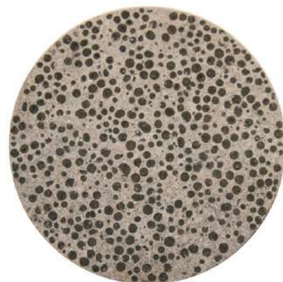
Fig 84 : Self healing concrete
